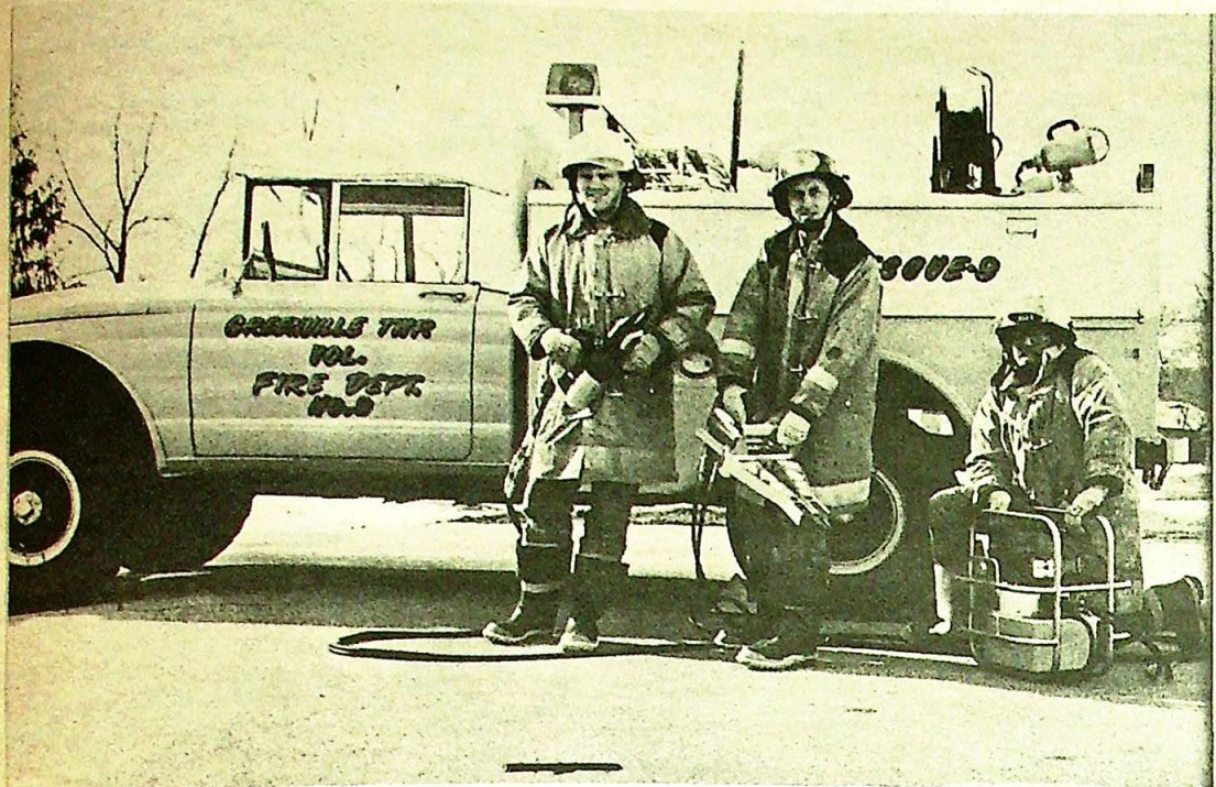
The Greenville Twp. Vol. Fire Dept., recently purchased the AmKus Rescue system which includes a 4 cylinder Briggs & Stratton power unit, a 20,000 lb. spreader and a 60,000 lb. cutter. The fire department was able to purchase the rescue equipment by having bingo games, a gun raffle, chili dinner and benefit auction, plus $3000.00 from the trustee. The equipment was delivered in January of this year, and since then, has been used on one accident. Pictured from left to right are: Jerry Burkhart, Captain Bob Allen, and Steve Simpson.
