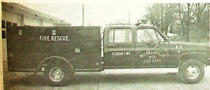
The McCordsville Fire Department purchased a 1986 GMC 1-ton, 4-wheel drive truck with dual wheels and a crew cab. The department designed their own utility bed with all the compartments going straight through from side to side.
