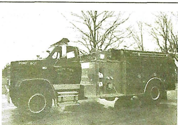
1000 Gallon - 1000 GPM Pumper
