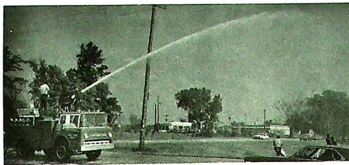
Gary FIRE TASK FORCE Squad 225 with Task Force Tip operating at 400 gpm with TFT maintained 100 psi nozzle pressure. Good stream, good reach for the flow rate (which under fire conditions would be whatever flow available). For purposes of the tests shown, flow from the hydrant through a flow meter was gated down to simulate short water supply.
