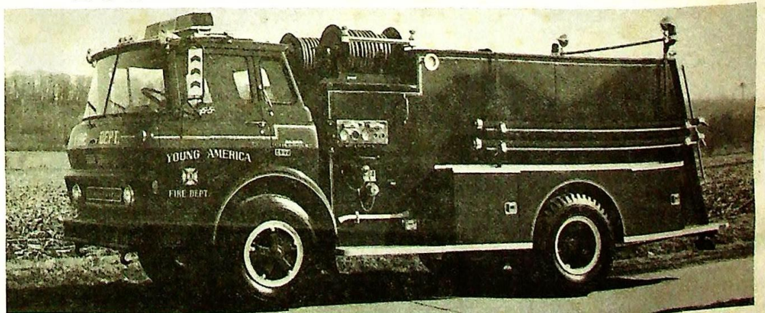
This apparatus, built on a Chevrolet Chassis, features a Hale CBP Pump, 1500 gallon booster tank, 700' capacity of 1 1/2 hose, side and rear compartments.
