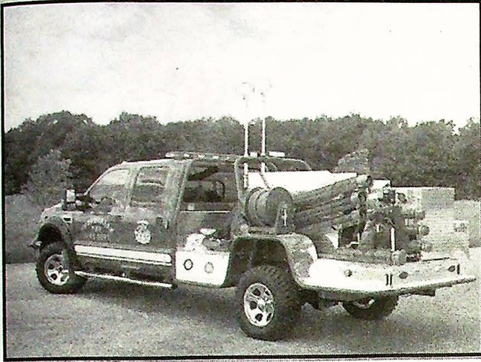
Thorncreek Township Fire Department in Whitley County, Indiana, recently took delivery of a Fast Attack Brush Truck from Wildfire Manufacturing, Inc. This Ford F350 crew cab features a 220 gallon custom water tank, 500 gpm Darley diesel pump, safety jump seats, emergency and scene LED lighting, and a navigation system. - submitted by Anisa Waterhouse, Wildfire Manufacturing, Inc.
