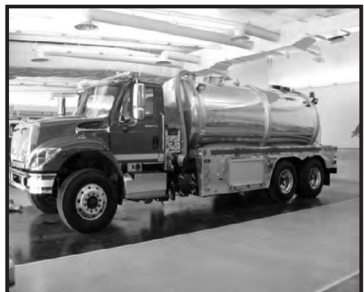
2013 Int./E-ONE Water Master 330 hp, 500 gpm, 3500 Gallon
