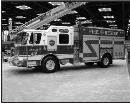
2012 E-ONE E-MAXRes/pumper 450 hp, 1500 gpm, 750 gallon water
