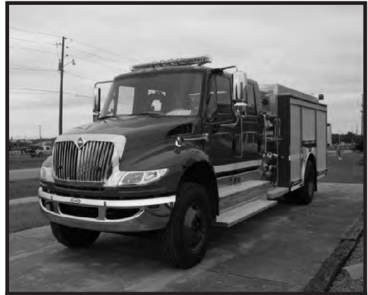
2013 Int/E-ONE Rescue Pumper 330 hp, 1250 gpm, 1000 gallon
