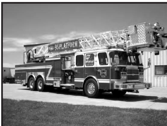
2012 E-ONE 95' HP RMP 500 hp, 2000 gpm, 500 Gallon Water
