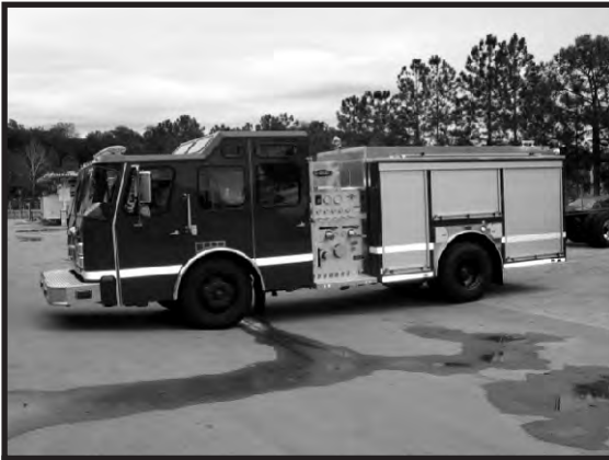
2013 E-ONE Rescue Pumper 350 hp, 1250 gpm, 780 gallon water
