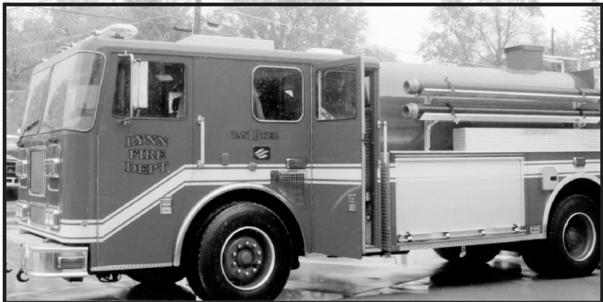
(Pictured above) – LYNN VOLUNTEER FIRE DEPARTMENT'S NEW TANKER. It is a 2001 Seagraves four man cab. It holds 2000 gallons of water and pumps 500 gallons per minute. It has a new body and tank and was built by McGinly from Lebanon, IN.
