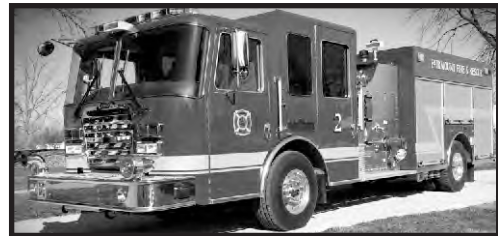
The Fairmount FD recently put into service a new KME engine. The 6 man custom cab has a 1500 GPM pump with 1000 gal. of water and 20 gal. foam tank.
