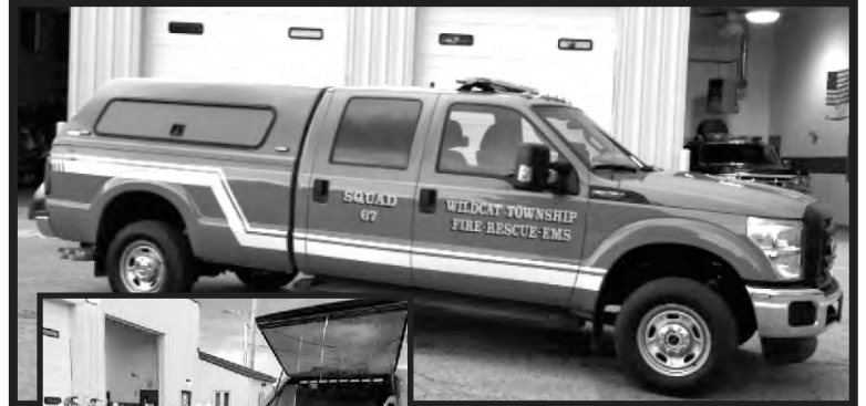
Wildcat Twp. VFD of a new squad recently put in service by the department. The 2015 Ford F-350 4x4 is equipped with a roll out tray to hold extrication and rescue equipment. It also holds a first responder bag and
