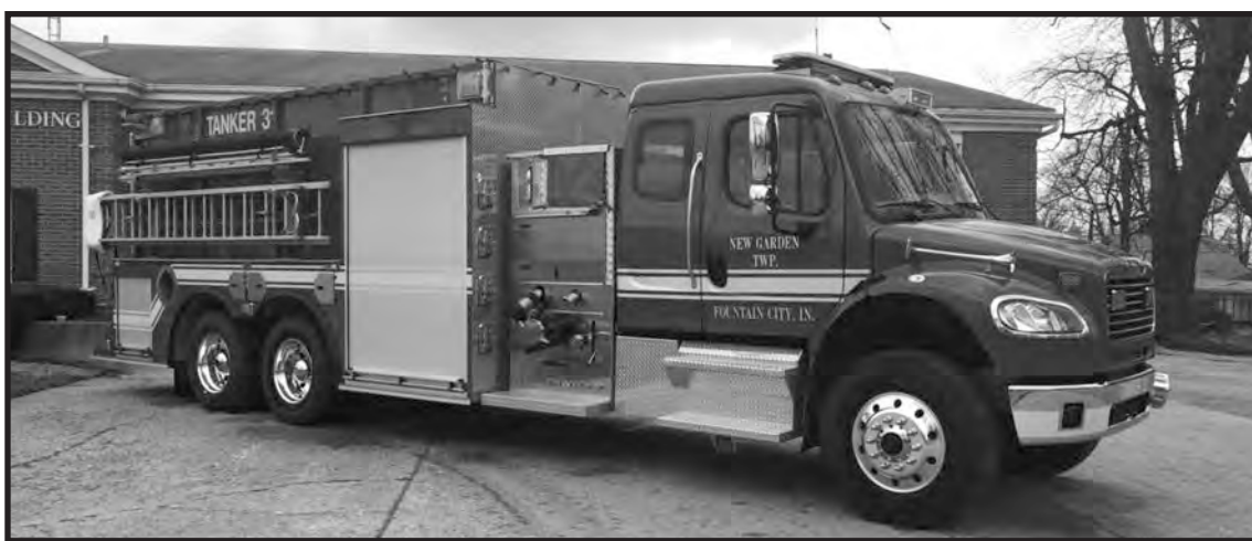
Fountain City Fire Department has two new trucks – a 2016 freightliner 3,000 gallon tanker 1250 gpm pump. Also a 2019 Dodge Ram 1/2 ton crew cab equipped with grain bin rescue tools, also serves as a command truck. Both vehicles were built by Warner bodies in Elwood, Indiana. – submitted by Shane Shroyer
