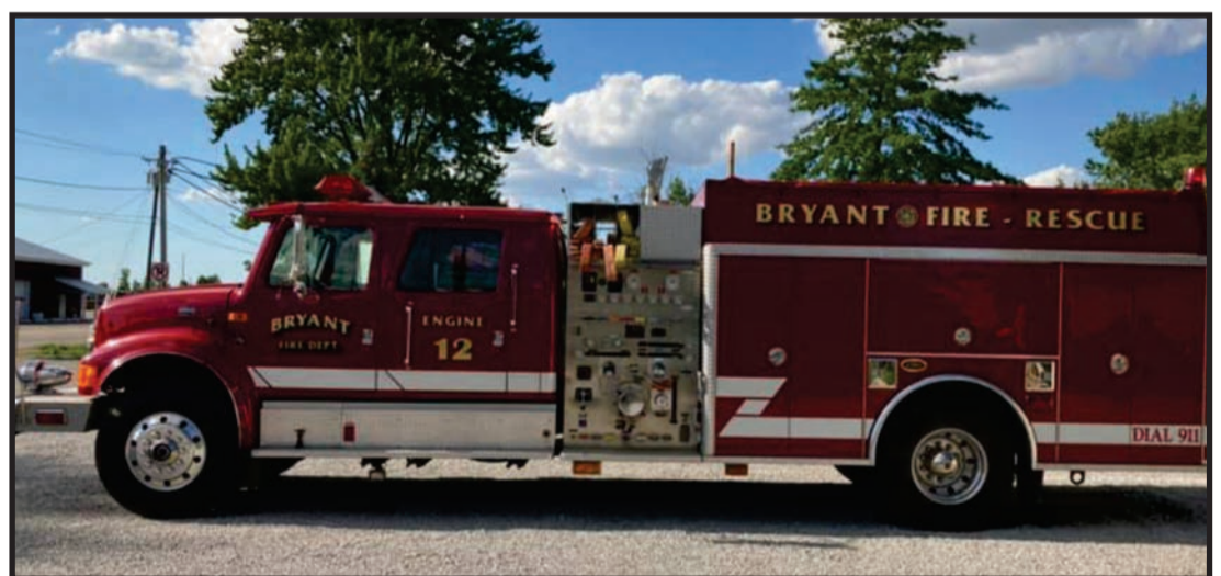
The Bryant Volunteer Fire Department new Engine 12. They purchased it from the Montezuma Fire Department in Montezuma, Ohio. It is a 2000 IH KME fire engine. It has a 1500 gpm pump and a 1000 gallon water tank. It also came with a full compliment of fire hose including 1 3/4" hose and Nozzles, 2 1/2" hose, and 5' supply hose. It also included some miscellaneous equipment including floating strainer, negative pressure fans, and stream light box lights.
