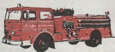
5-man canopy-type cab with removable section in top for easy access to engine; dual ignition; 500 gal. booster tank; four large side compartments; two large rear compartments.
