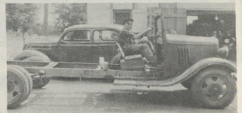
The chassis from an old school bus which was used to construct Waynedale Fire Department's first motorized tanker. The complete construction project was done by volunteers.
