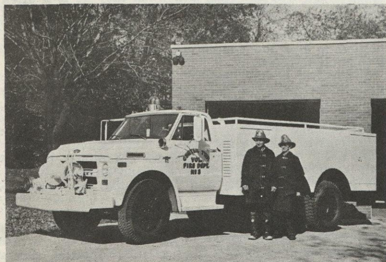
Assistant Chief Bill Kolash pictured above with Pat Kepplin worked many long and hard hours to construct the new tanker which was recently presented to the department. It features a Chevrolet Chassis with a front mount winch and is capable of carrying 1800 gallons of water.
