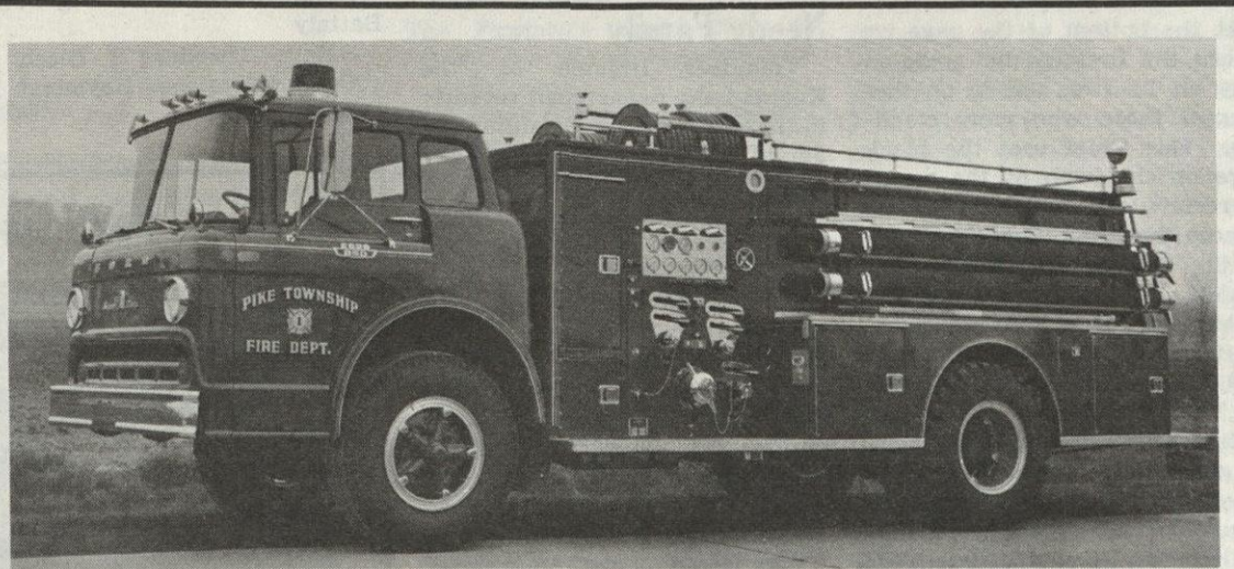
The above Midwest pumper is the first unit of its kind delivered to a fire Department in Marion County, Indiana. This unit is equipped with a 1000 GPM Hale Fire Pump, and an Allison MT-42 automatic transmission.
