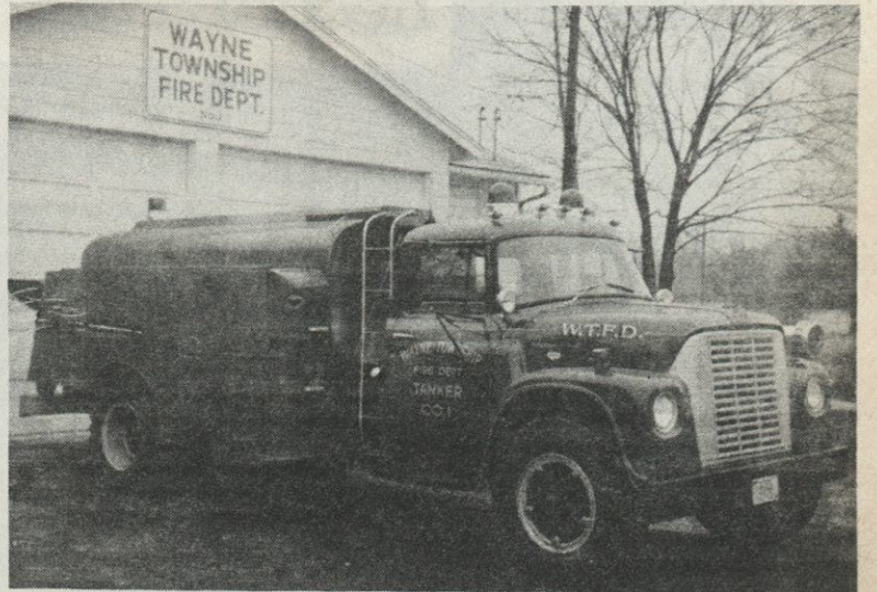
This truck is an International Harvester 1970 chassis with 1350 gallon capacity. It is Dual Frequency - Radio Equipped. It features 3 - 360 degree red light beacons, two forward and one aft.
