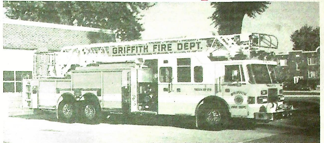
On September 15, 1998, the Griffith Fire Department took delivery of a 1998 Pierce Lance Quint. The new Ladder 218 replaces a 1964 Maxim and is assigned to the Central Station. This unit has 105' rear mount aerial. The pump is 2000 gpm Waterous and has a 500 gallon tank. The truck is powered by a Detroit Diesel Series 60 engine. The wheel base is 229.50 inches. The unit features the All Steer System. The cab seats six and is air-conditioned.
