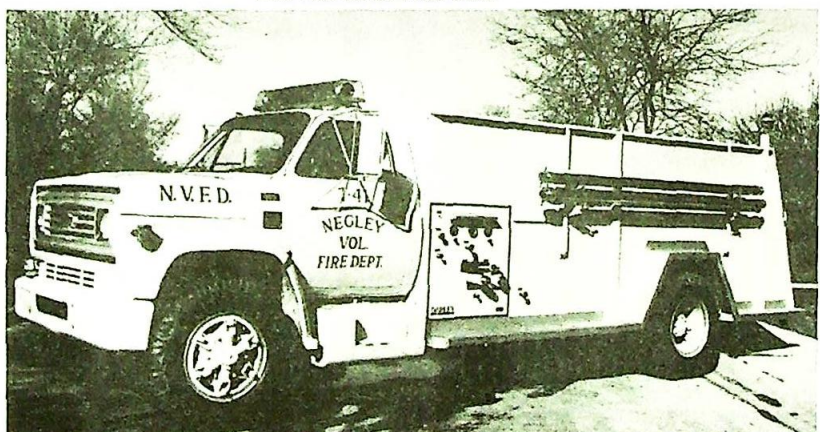
Negley, Ohio recently took delivery of this 1750 gal. tanker, complete with the famous Darley HM 350 pump. The chassis is a Chevrolet C65 with a 427 cubic inch engine.
