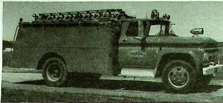
Tanker No. 3, built by members of the department in 1963. Carries 1100 gals. of water with a 300 gpm power take-off pump.
