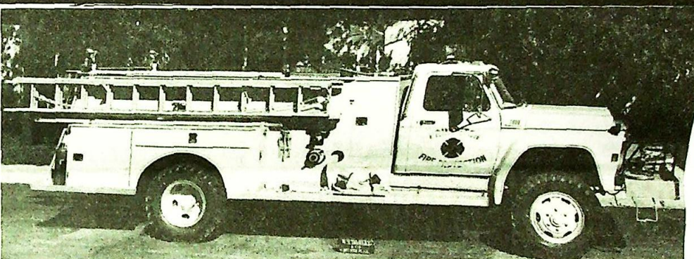
This sleek multi-use pumper for Princeton, Ill. has a 500 gal. tank and two pumps, a 750 gpm MODEL S 750 and an HM 350 PTO pump for pump and roll operation. Note the 6 foot booster lines on the front platform for fighting grass fires, etc. The chassis is a Ford F600 4x4 all wheel drive.
