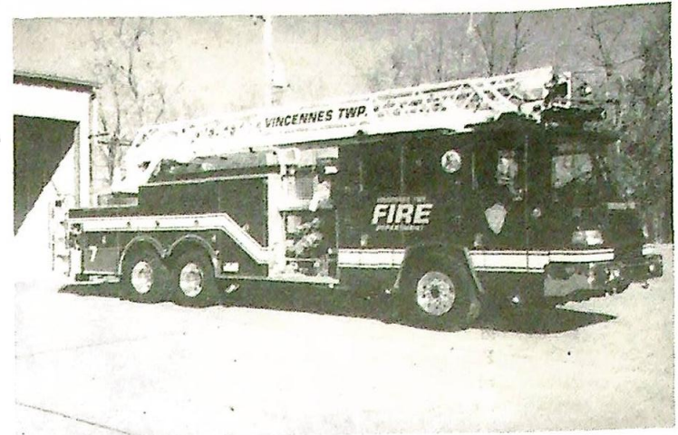
The Vincennes Township Fire Protection District, Indiana recently took delivery of a Pierce 75 foot heavy duty ladder. The unit is equipped with a 500 hp engine, 2,000 gpm Waterous pump and a 500 gallon poly tank.
