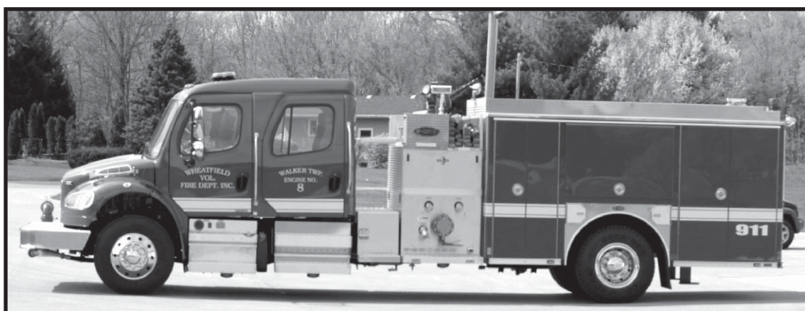
Wheatfield VFD has received a new E-1 Pumper on a Freightliner chassis. It has a 1600 GPM pump with a 1000 gallon poly tank.
