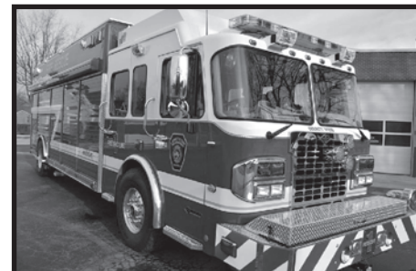
Lafayette Rescue 1 - A 2015 Spartan Metro star chassis with Hackney body, 6000psi Scott revolve air cascade, Genesis rescue tools with rear and forward connections, generator, light tower. High and low angle rescue capabilities Warn winch.
