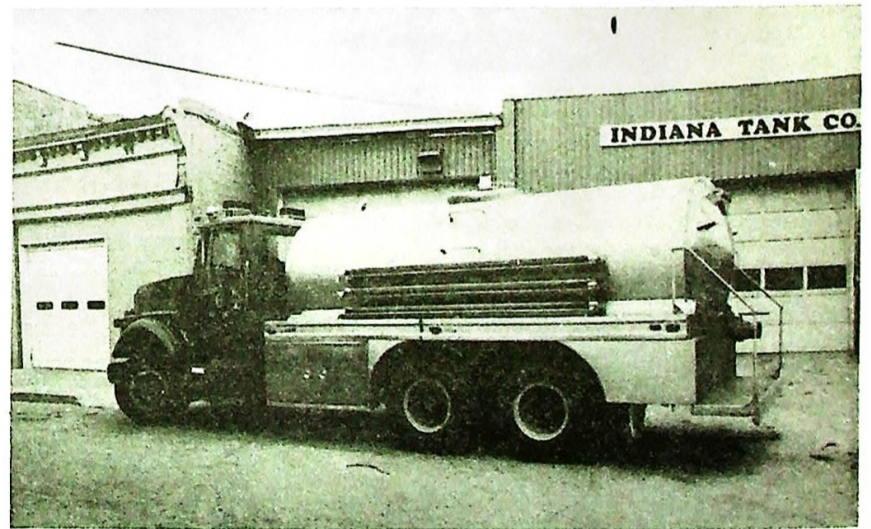
3,000 GAL. STAINLESS STEEL TANKER
