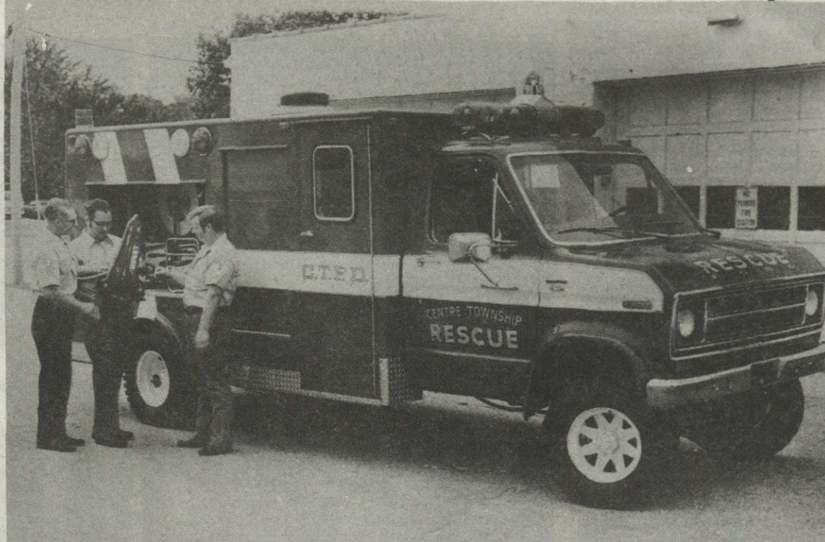
NEW RESCUE RIG - Members of the Centre Township Volunteer Fire Department, South Bend, examine equipment on their new rescue truck. From left are Dave Mikel, assistant chief; Dale Murphy, Jr., training officer, and Lamar (Red) Locke, chief. The truck, built on the frame of a Ford one-ton chassis, has four-wheel drive, 250 gallon of water and 20 gallon of foam, and a three K.W. generator. Red light in top telescopes sixteen feet from ground with four quartz to light up the working area, and carries tools for many kinds of rescue work.
