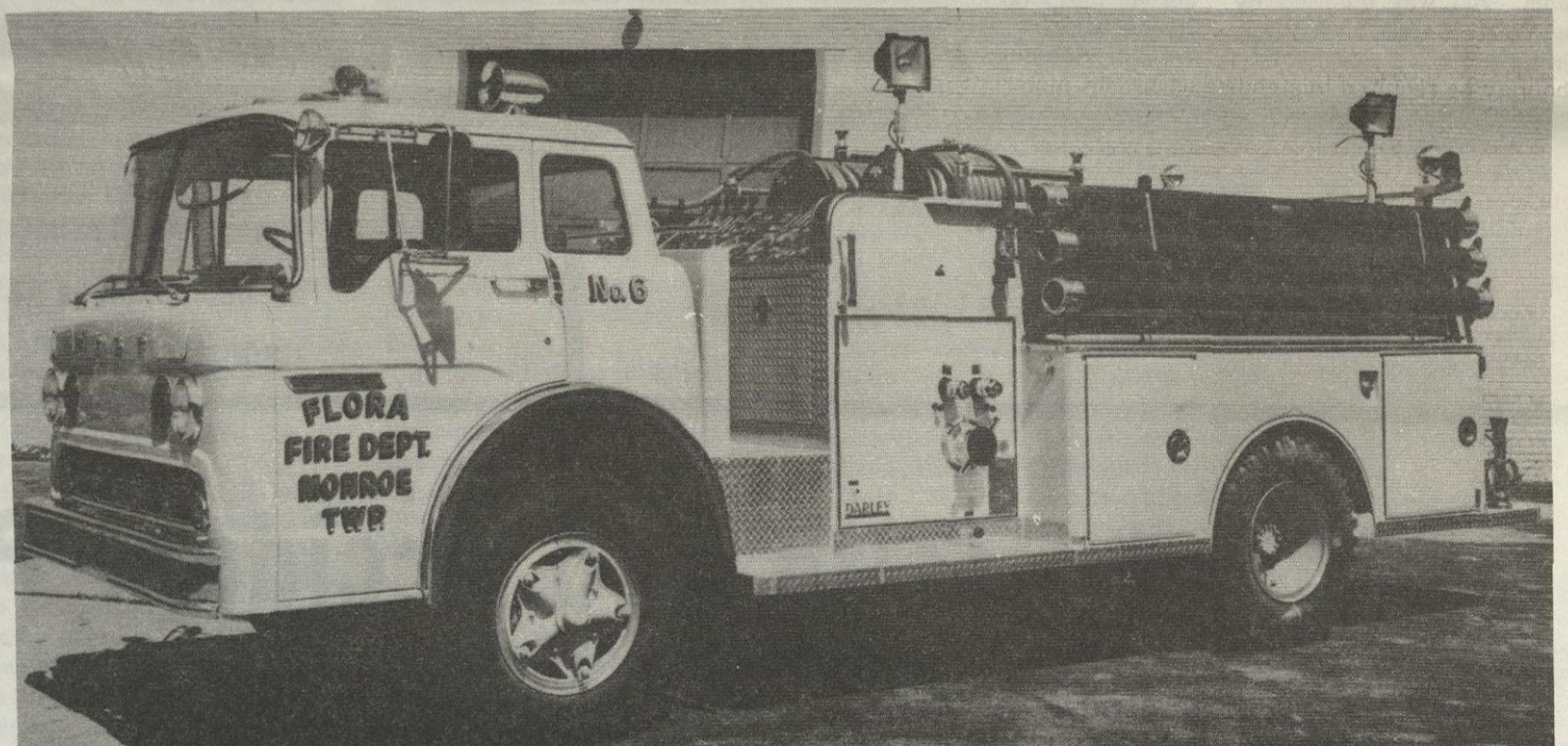
This Top Console model for Flora, Ind. carries an $1000 2 stage midship pump and a 750 gallon booster tank with an M.C. lighted tank gauge. Note the two 500 watt quartz floodlights.
