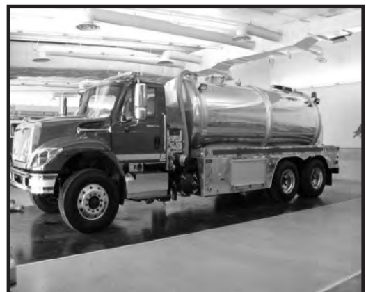
2013 Int./E-ONE Water Master 330 hp, 500 gpm, 3500 Gallon
