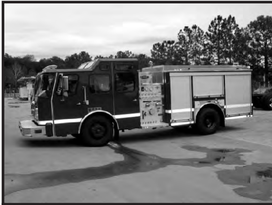
2013 E-ONE Rescue Pumper 350 hp, 1250 gpm, 780 gallon water
