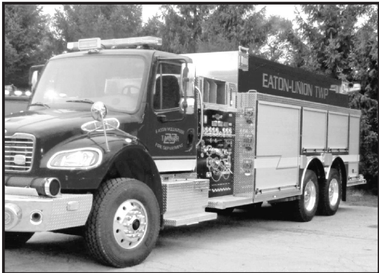
On September 14th the Eaton/Union Township Volunteer Fire Department received their new tanker. It is a Rosenbauer Freightliner with a 3000 gallon 1250 gpm pump.
